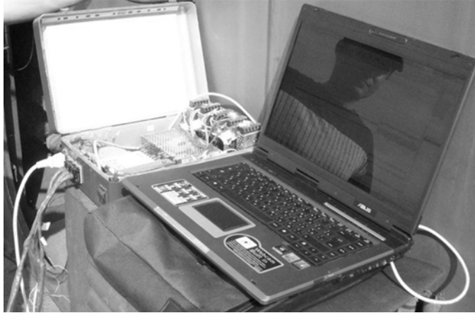
Fig. 8. Tension station with 32 information channels.
